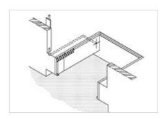
In the framework of the preparation for assembly works, we can supply steel frames for the fixing of the leveller well in advance for concreting.
